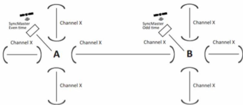
Figure 3 - Two sites using the same channel for both PtP and PtF connectivity. The two SyncMasters ensure inter/intra site functionality.
